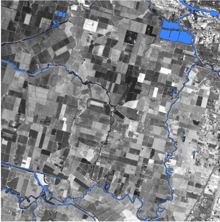
Figure F10G: Map of Open Water (Light Blue) Using a Threshold (-200) on TC1 Values.
