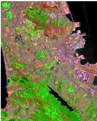
Output raster set (warped and reoriented to the UTM coordinate system), displayed with UTM grid tick marks along the border for emphasis.
