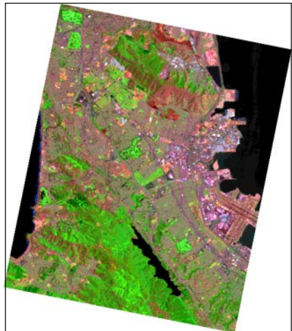
Output raster set in the NAD27 / SPCS27 California Zone 3 (ftUS) coordinate reference system.
