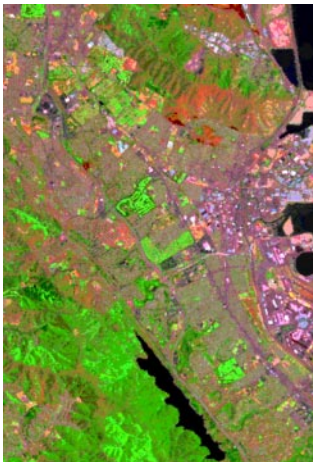
Output rasters in State Plane 1927 coordinate system, with extents specified in the Extents panel. Compare with image on page 6.
