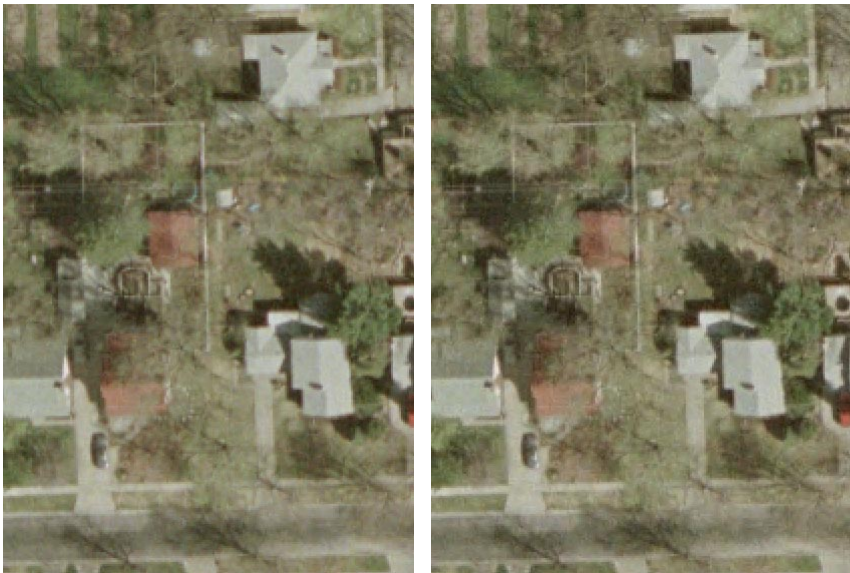
The original downloaded TIFF file (left) is compared at 2X with the purchased MrSID 10:1 compressed file. Both are directly displayed (not imported) in their native format.
