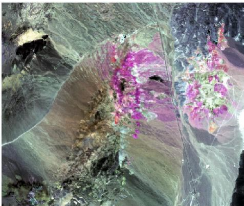
Bands 172 (1.989 \mu\text{m} ), 187 (2.139 \mu\text{m} ), and 202 (2.288 \mu\text{m} ) displayed respectively as R, G, and B. This band combination highlights the hydrothermally altered rocks in the Cuprite scene and distinguishes different types of alteration.
