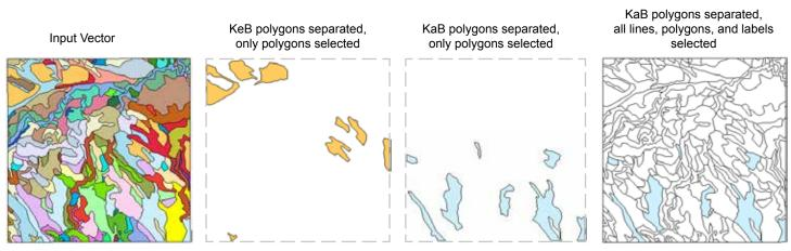
The output objects shown above are among the 48 vector objects created when polygons are separated by soil class, which involves a total of 48 attribute values in this example. Styles that have been specified by attribute in the original object are transferred to each of the output objects and the last used style is assigned by default when the new vector objects are displayed.
