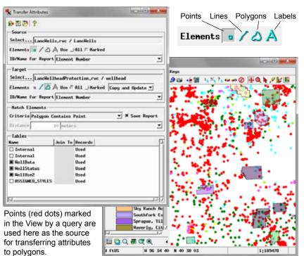
pushbutton to choose a vector, CAD, or shape object to use as the source/target for the transfer. The file and object name of the selected object is then shown in the text field to the right of the pushbutton. The relevant Elements icon buttons are activated automatically according to the element types available in the object. If more than one element type is present, turn on the icon button for desired element type.
