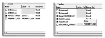
Turn on a toggle button for each source table in the Name column you want to transfer to the target. If the field for a table in the Join column has a white background rather than gray, it means that one or more tables with the same structure as the source table (number of fields and same field types) exists in the target object. Left-click in the Join To field to show a menu from which you can choose a table to write the records to, or choose None to copy the source table to a new target table.
