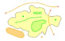
Attributes from the source polygon (yellow) would be transferred to any of the contained elements (green) but not to the orange elements that are partially or completely outside the polygon boundary.
