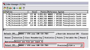
In the illustration above the individual input LAS files are being reprojected from Pennsylvania State Plane coordinates to UTM coordinates (set using the Output CRS button).
