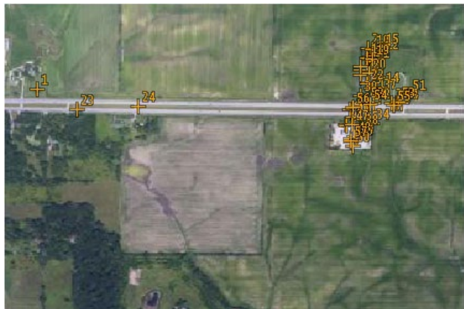
Keypoint Matching (on full-resolution image): 57 control points.
