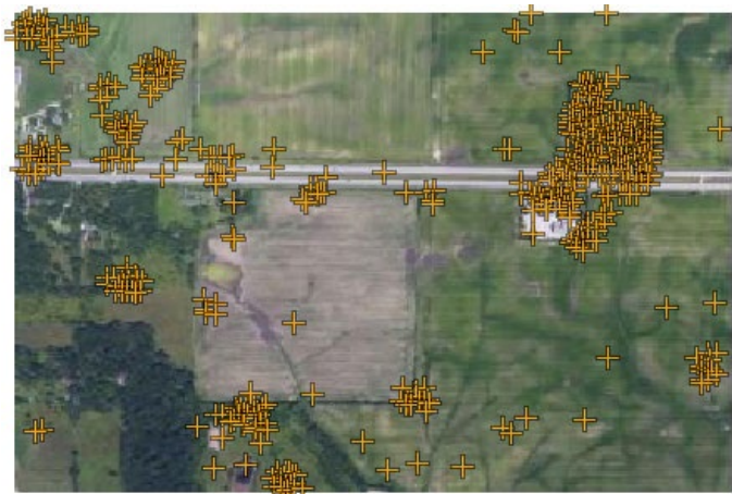
Automatic (keypoint matching on reduced-resolution pyramid tier followed by cross-correlation): 512 control points.
