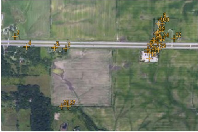
Estimate from Single Point (keypoint matching on reduced-resolution pyramid tier): 27 control points.
