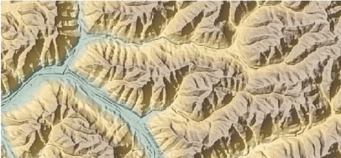
5 x 5 Voltaerra/Unsharp sharpening filter applied only to the shading raster layer, producing a crisper image of the terrain.
