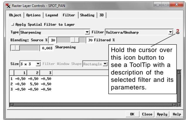
Use the controls on the Raster Layer Controls window's Filter tabbed panel to choose a category and filter and set the specific parameters for that filter. You can quickly turn filtering on or off using the toggle button at the top of the panel.
