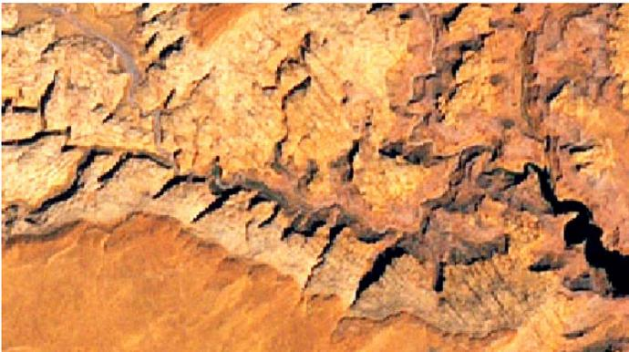
Left, color satellite image (15-m cell size) of desert area with exposed rock layers exhibiting northwest-trending vertical fractures. Right, same image displayed with integrated filtering
