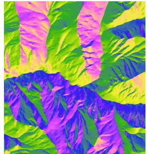
Aspect raster displayed with cyclic uniform perceptual contrast color palette with matching colors at either end. Note smooth transition between colors for northwest and northeast-facing slopes on south wall of major valley.
