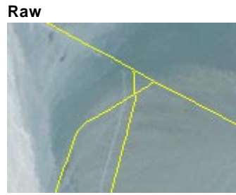
Road intersection, elevation 1003 m. Road offset of ~95 m corrected in orthorectified image.
