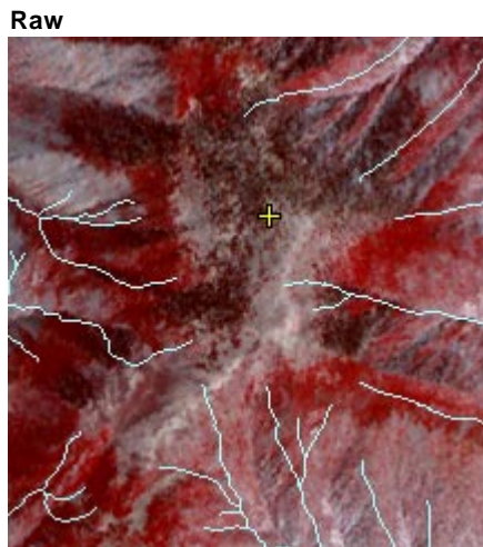
Streams and mountain peak (cross), peak elevation 3380 m. Stream and summit offsets up to 283 m corrected in orthorectified image.
