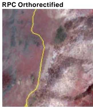
Road, elevation 3130 m. Road offset of ~110 m corrected in orthorectified image.
