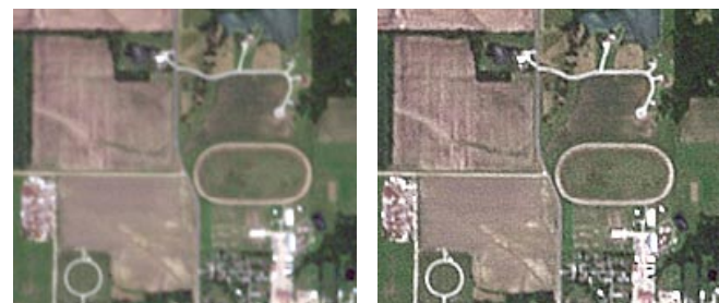
Above, Filter View window displaying the result from applying the Volterra/Unsharp sharpening filter on a color image (RGB separates). The boxed area is shown at 1X for the input image (below left) and for the filtered result (below right).
