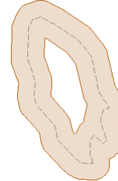
Border buffer (outer ring + inner ring) from a polygon (dashed gray line).
