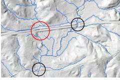
This bare-earth LIDAR DEM was edited prior to distribution to breach manmade structures (highway embankments and bridges) crossing major streams (black circles). Some smaller drainages are still blocked (red circle), causing Watershed flowpaths to be diverted by these features.
