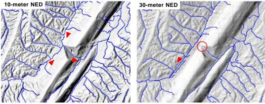
Watershed flowpaths computed from 10-m NED (left) and 30-m NED (right). In the left illustration a stream correctly breaches a major ridge (flow directions shown by red arrowheads). The 30-m DEM (right) has insufficient resolution to accurately represent the true elevations at the upstream end of the narrow, steep-sided gorge (red circle), diverting watershed flowpaths to an incorrect lowerelevation outlet. Local editing of the spurious cells in the 30-m DEM can remove the blockage.
