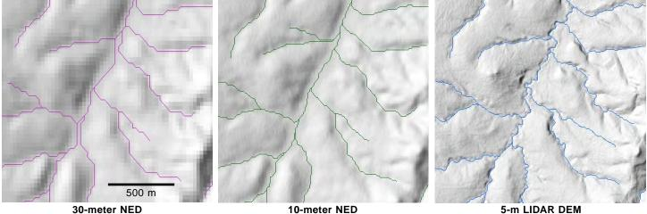
Comparison of flowpaths computed by TNTmips Watershed process from DEMs of differing cell size and quality for a lowrelief area in northern Louisiana. Flowpaths (colored lines) are overlaid on shaded-relief images computed from the respective DEM. Cell values in each DEM are integer feet; maximum
