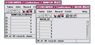
Flowpath Hydrologic Connectivity: Each flowpath line can flow into only one downstream stream line; the ID number of that line element is recorded in the DOWNFLOW table for each line. The BASINS table is only created when basins are computed along with flowpaths; it records the ID number of the basin polygon in which each stream line lies. This table has one record for each basin, with each basin record attached to one or more of the stream line elements.
