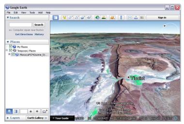
Google Earth display of a tileset stored in a KMZ file. This tileset consists of 2383 tiles at 7 zoom levels. The KMZ file containing this tileset is about 125 MB in size.
