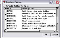
The Database Settings option on the right mouse-button menu for a geometric element (left) opens the Database Settings window (above). This window provides a Default Tables to Open checklist
