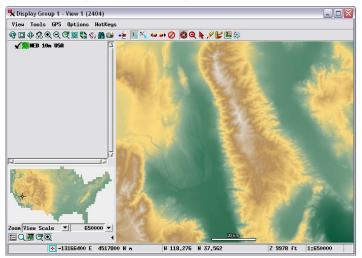
View zoomed into a portion of terrain surface layer using the NED 10m USA web terrain tileset hosted at microimages.com. The surface is rendered above by color-coding elevation values using a color palette selected in the Surface Layer Controls window. The illustrations below show two alternative renderings of the same portion of the terrain: relief shading (left) and combined shading and elevation colors (right).
