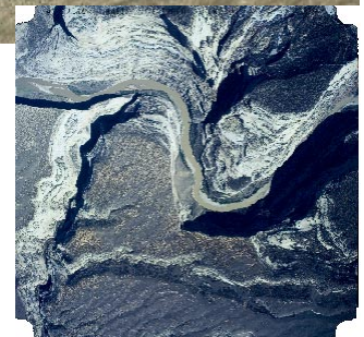
Right, unrectified color aerial photo of an area about 3 km wide featuring a deep canyon (over 300 m local relief) in northwest Colorado, USA. Above, the photo raster after georeferencing (with over 450 control points) and reprojection using the Thin Plate Spline model. The photo is overlaid on an orthoimage of the area. The red lines superimposed on the photo show the resampling result for a set of originally orthogonal grid lines matching the extent of the photo. These lines emphasize the varying changes in geometry of the photo resulting from the reprojection.
