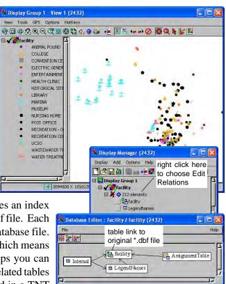
The above tree diagram shows the relationships between tables formed when a shapefile is selected for direct display in the TNT products. The LegendNames table and style Assignment Table are created automatically in TNT when a shapefile is selected if it has a \*.avl file with this information. This information is stored in the same-named \*.rlk file.
