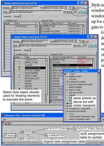
Style assignment for shapefiles presents all element types in a single window. Make sure the correct element type is selected in this window (for this example, points). To use the styles already set up for drawing the shapefile, click on the Styles button and navigate to the Styles subobject under the shape object that is selected
