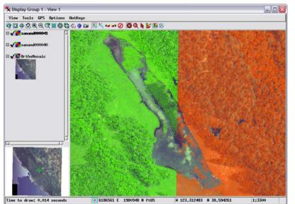
Detail of two linked LAS LIDAR shape layers (green and orange point clouds) displayed over a reference 1-meter color orthoimage (shown to the right at the same scale for comparison). The gaps in the point clouds are due to missing LIDAR returns from the largely algae-covered pond surface. These LIDAR points, acquired and
