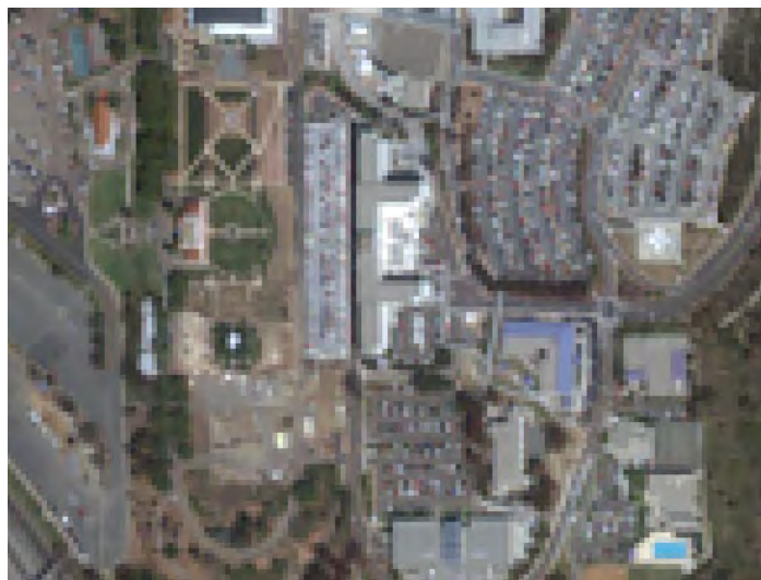
Natural-color RGB display of 4-m resolution multispectral bands from a portion of an IKONOS image bundle. Natural-color Multiresolution Fusion results for this area using two color fusion methods are shown below.
