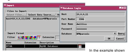
here, TNT spatial data on a PC running Windows XP is linked to a database in a MySQL database server residing on a PC running LINUX.
