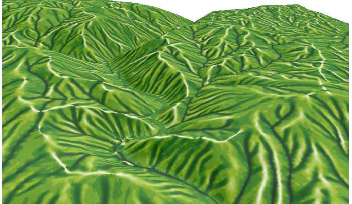
**Plan (contour) curvature** raster produced by the SURFCURVE script, displayed with color palette over the terrain. Positive values indicate convex-outward surfaces.
