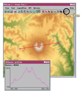
Profile from a digital elevation model raster. The vertical graph axis is labeled with the minimum and maximum cell values along the profile line. The horizontal axis is labeled with the endpoint positions in raster coordinates (column, line).
