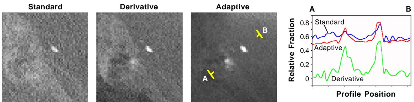
Comparison of matched filtering results for a small part of the Cuprite, Nevada AVIRIS scene using the wavelength range 1.98 to 2.5  $\mu\text{m}$ . The target signature is an image spectrum for the mineral alunite. Only the brighter of two small concentrations of alunite is evident in the standard matched filter fraction image. The weaker concentration is barely identifiable in the derivative matched filter image against the still-noisy back-
