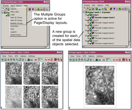
When multiple groups are added to a display layout, groups are automatically tiled and have no specific attachments.
