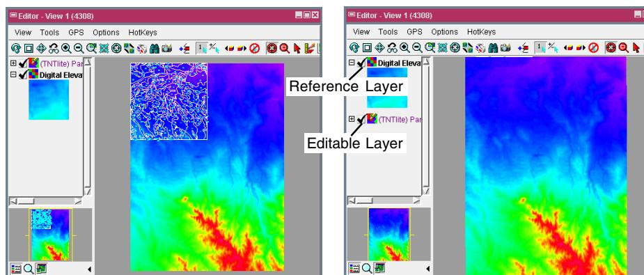
The reference layer is automatically added below the editable layer when Add Reference Layer Below Edit Layer button is toggled on.
