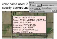
A multiline DataTip specified in a virtual field for a single layer can contain the color specification for its background, but here (above left and right) it is specified in the prefix field for the DataTip in the Layer Controls.
