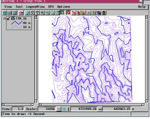
This Group View was opened when the TIN object was selected. In this case, the last-used display parameters specify that the TIN object selected be automatically converted to and rendered as contours at two specified intervals, which were set on the Contours panel of the TIN Layer Controls.
